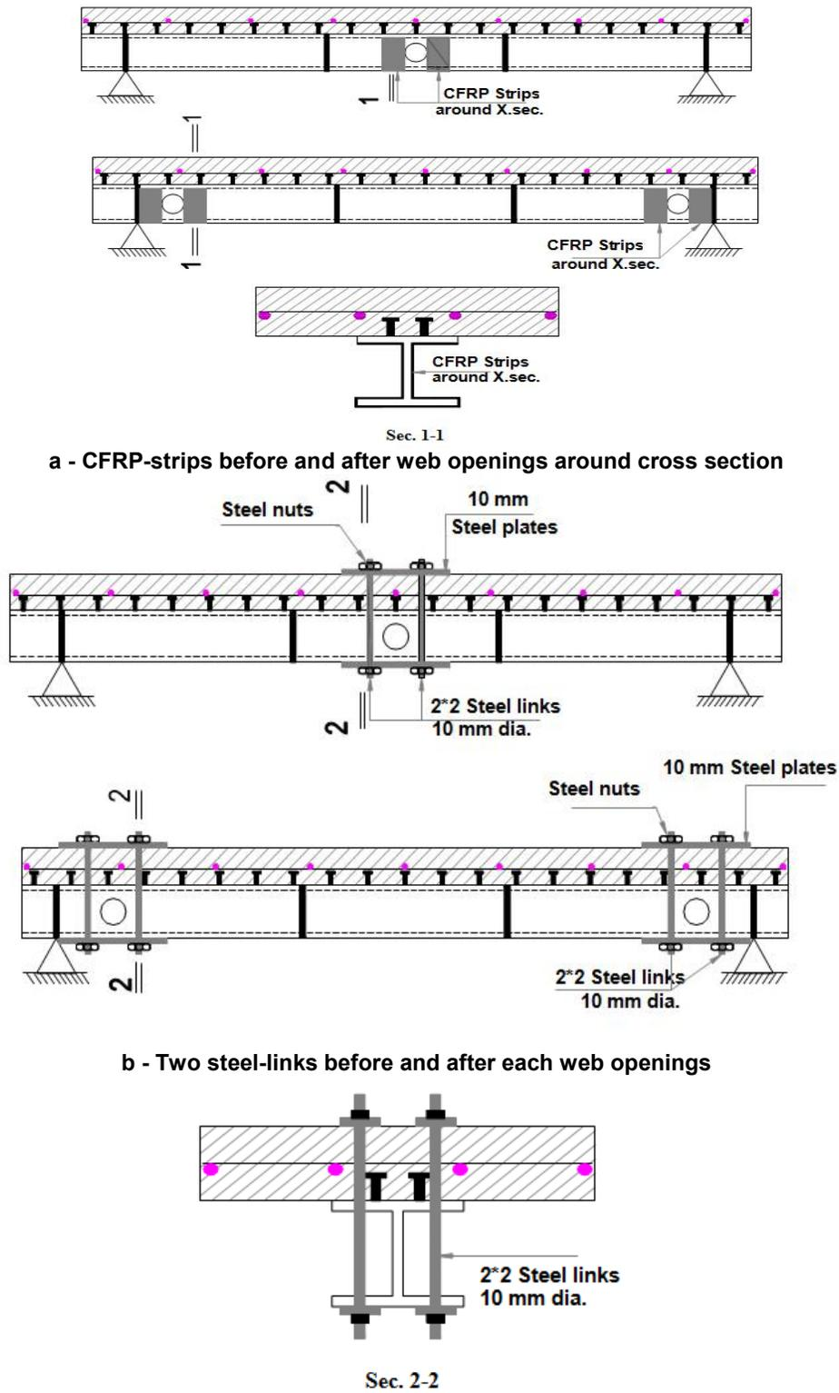
Fig. 4. Description of different strengthening techniques (Note: all dimensions in mm)
