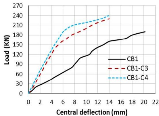
Fig. 9. Effect of number of CFRP layers on load-deflection relationships
