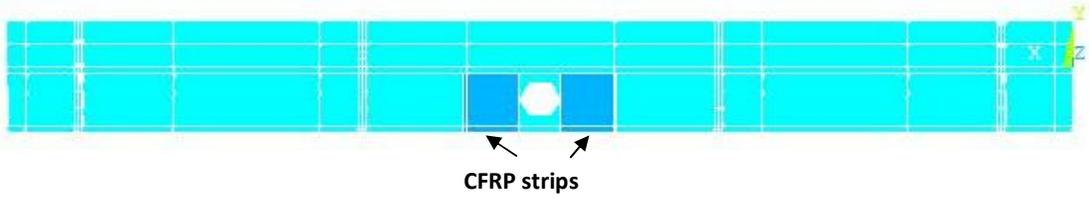
(e) Composite beam strengthened with CFRP strips around openings
