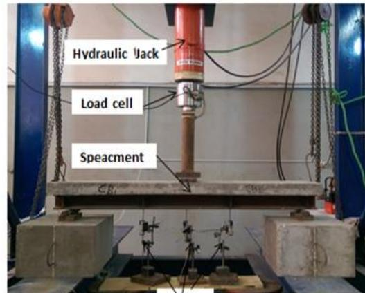
**3a. Central one-line load across the width of the concrete slab**
