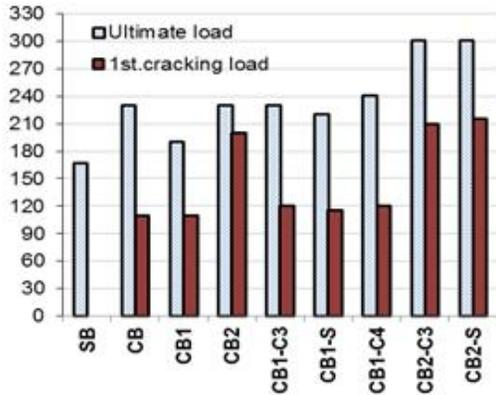
Fig. 11. Cracking and ultimate loads comparison for all tested beams
