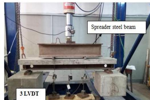
**3b. Two-line loads across the width of the concrete slab****Fig. 3. Test set up & LVDT locations**
