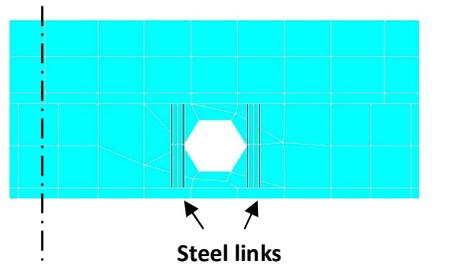
(f) Composite beam strengthened with steel links
