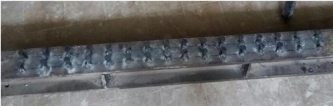
a- Shear connectors with 10 mm diameters welded above the compression flange
