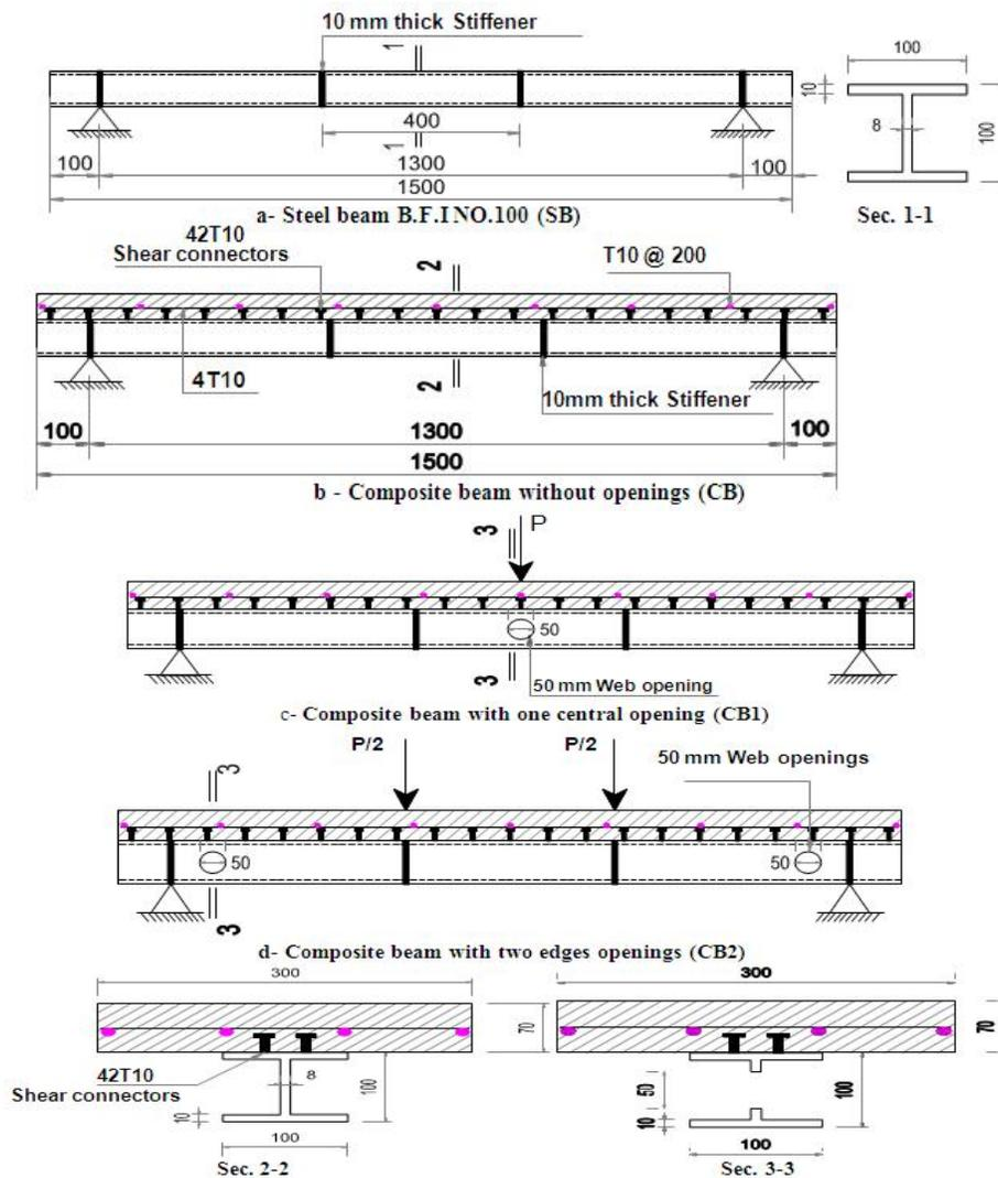
Fig. 2. Longitudinal and cross section details of beam specimens (Note: all dimensions in mm)
