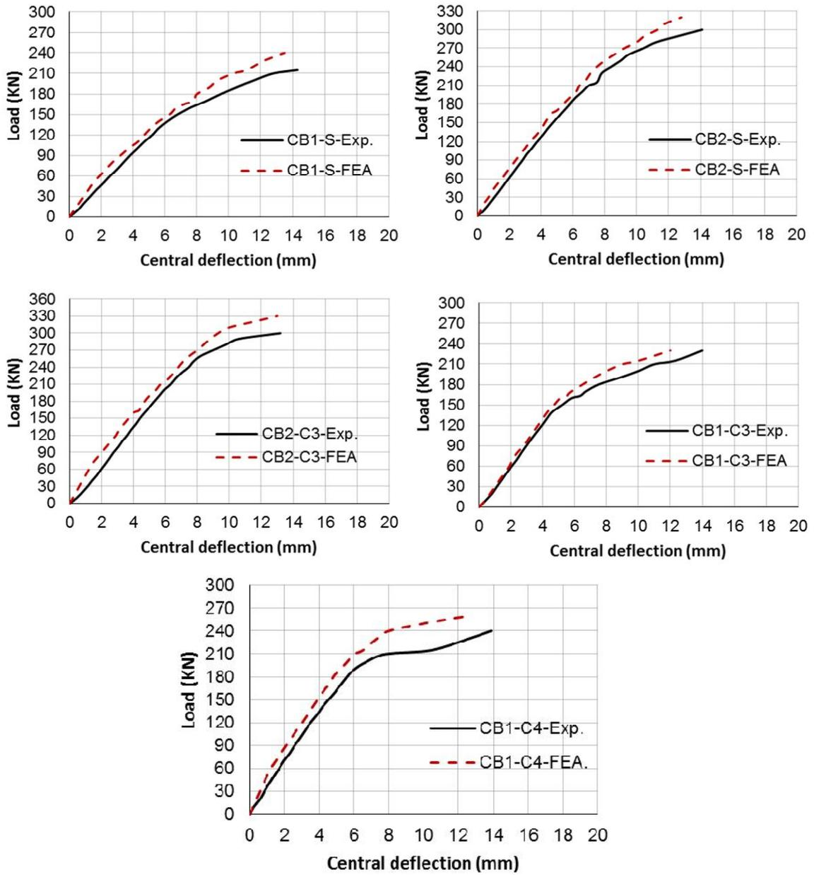
Fig. 18. Comparison of experimental and FEM load – deflection curves
