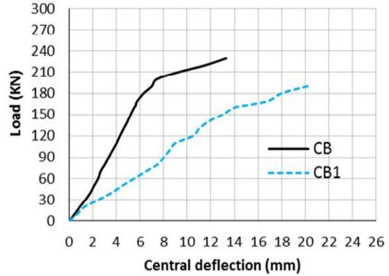
Fig. 6. Effect of web openings
