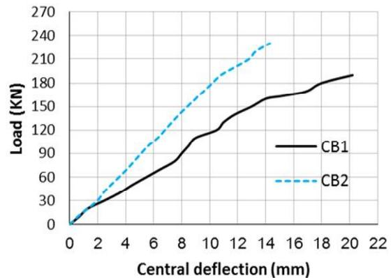
Fig. 10. Effect of location of web openings
