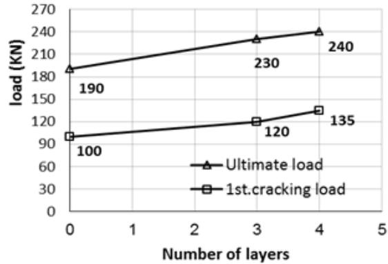
Fig. 12. Effect of number of CFRP layers on Cracking and ultimate loads
