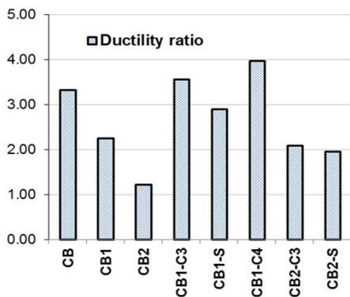
Fig. 15. Ductility ratio comparison for all tested composite beams
